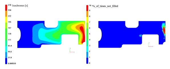
Fig. 5 Filling pattern in case of a deterministic study no air entrapments (left). Possibility to have an air entrapment in case of a geometry sensitive to race tracking (right).
