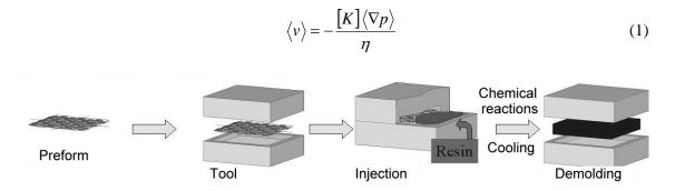
Fig. 1 Schematic showing the different stages of the RTM process.
